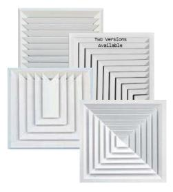
Louvre Faced ceiling diffusers are manufactured from extruded aluminium to BS 1474. Frames and all blade corners are mitred, welded and finished to give a superior appearance.
