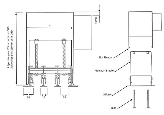
If the above slot widths do not match an existing diffuser, please confirm actual slot centres as the widths can be modified in production.
