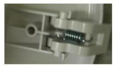
4-no clips snap shut when diffuser neck is pushed into the template hole. The clips bite the plasterboard to hold the diffuser in place.
