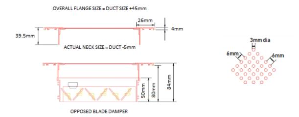
We can manufacture bespoke perforated grilles and powder coat to any BS or RAL colour within 5 working days.
