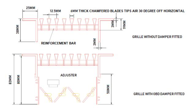
Standard 25mm flange can be cut down to 20mm on request.
