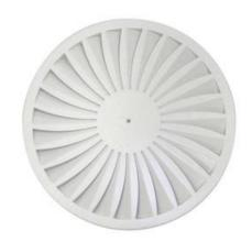
The Circular Flanged Swirl Diffuser has fixed spiral blades that create rotational as well as axial, tangential and radial air movement.
